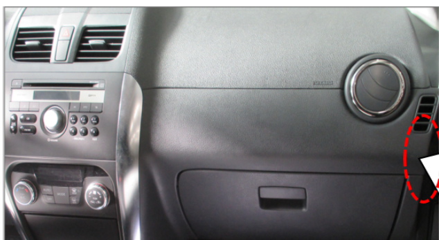
Location of the SX4 CVT Controller Assembly
